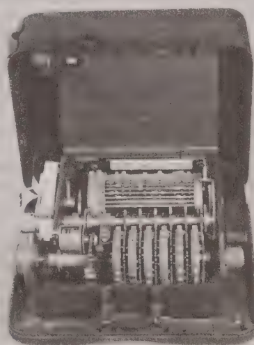
Figure 6: Hagelin design M-209 U.S. cipher machine used for tactical communications during World War II.
